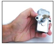
Using set-up key or the key the lock is now set to, turn the key CLOCKWISE 90° (1/4 turn) so the key is midway between its full locked and unlocked positions.
